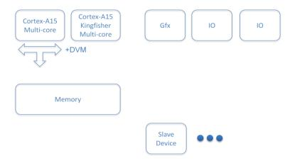
Figure 6 - ACE inner coherent logical view
