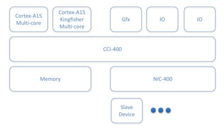
Figure 1 - Multiple coherent master system
