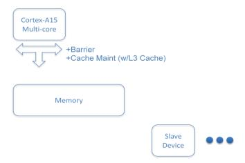
Figure 4 - ACE non-coherent logical view
